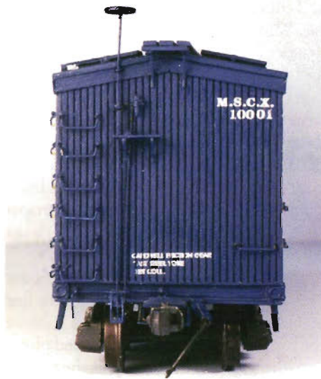
Above: This is the car's B-end, showing placement of the retainers, roof walk support with two braces, coupler lift bar, platform, brake staff bracket, and decals.
