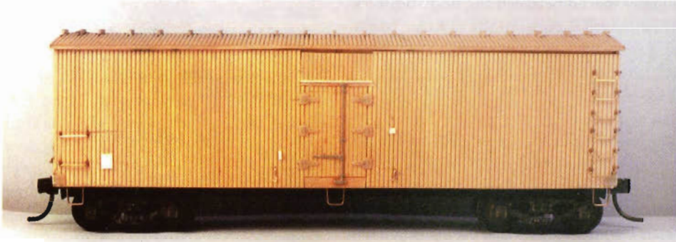
Above: The sides of the car were nearly finished at this point. Notice the kick board, header, drip molding, fill-in sheathing, grab iron placement, and the myriad other details included in the car. The roofwalk was yet to come.
