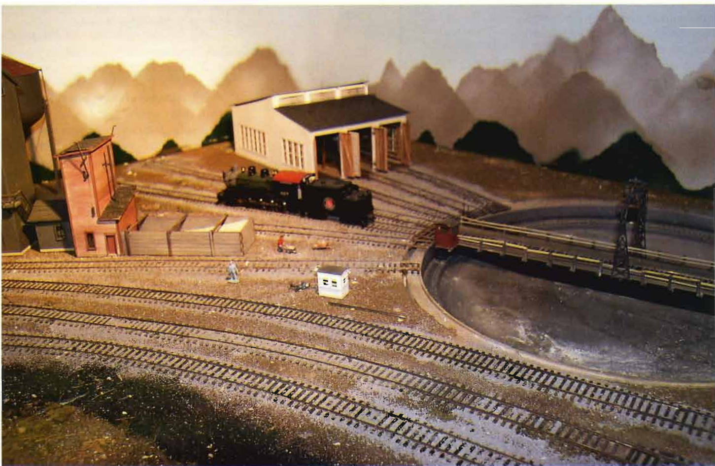
Above: This shows a three-way turnout, the siding, and the ladder in the yard. All these are powered by Tortoise switch machines and controlled by Digitrax DS 54 stationary decoders, wired though and match Larry's hand drawn sketches, although they were drawn for his former layout.
